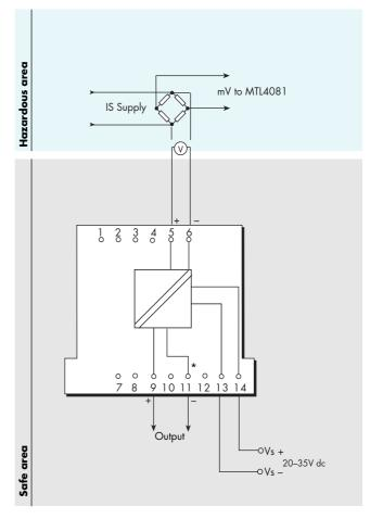
Note: output negative (terminal 11) is clamped to supply negative (terminal 13) through two series diodes
