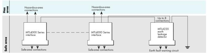
Note: some MTL4000 Series modules are multichannel and could require one connection for each channel.
