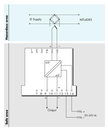
Note: output negative (terminal 11) is clamped to supply negative (terminal 13) through two series diodes
